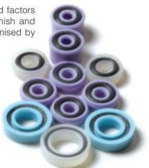
Surface finish also affects sealing ability. A rough finish creates a microscopic "line of sight" channels allowing a flow path through mating parts. When sealing gases with small molecules, such as, hydrogen, helium, or oxygen, a 2-4 RMS is highly recommended.
