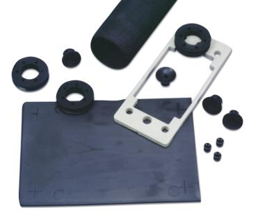
Conductive elastomeric seals aid designers by providing a component that can provide both environmental and electric sealing. Proper selection of the elastomeric binder is critical for environmental conditions, and proper selection of the metal filler is critical for galvanic capability to mating surfaces, and corrosion resistance.
